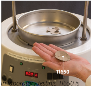
In laboratory testing, TI650 is proven to maintain material integrity, resistant to cracking, separation, and dusting when exposed to heat and vibration typical in vehicle applications.
